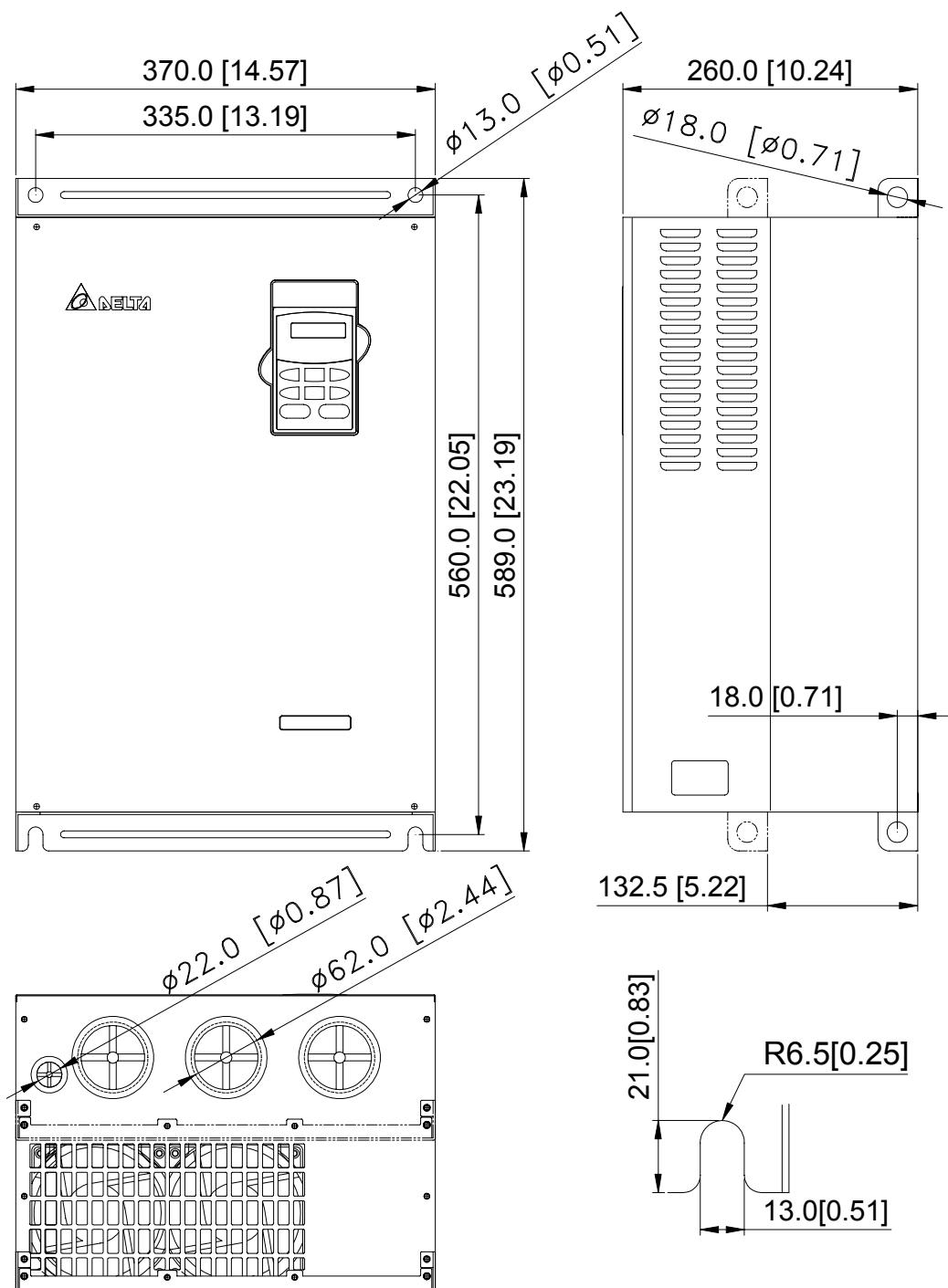
**Типоразмер Е1:** VFD300B23A, VFD370B23A, VFD550B43C/53A, VFD750B43C/53A
