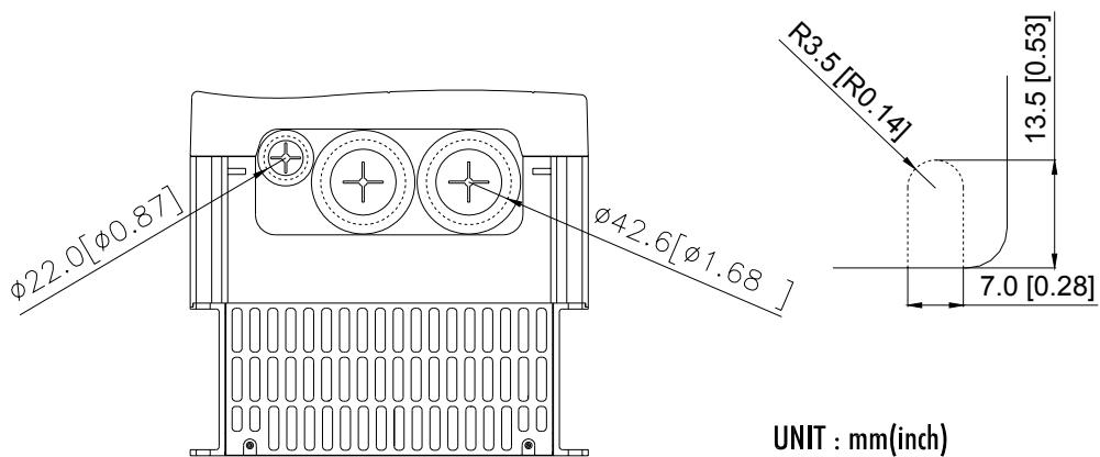
**Типоразмер D:** VFD150B23A/43A/53A, VFD185B23A/43A/53A, VFD220B23A/43A/53A
